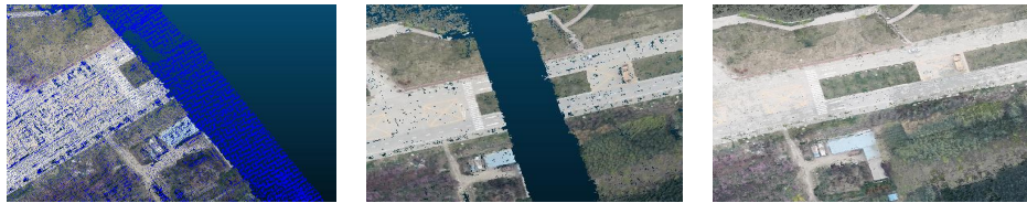
Fig. 7. Comparing reconstruction results in Different situations. The left cannot acquire submap’s relative transformation without the use of VGMM. The middle is a lack of center UAV image data with the use of VGMM. The right involves entire dataset with the use of VGMM.
