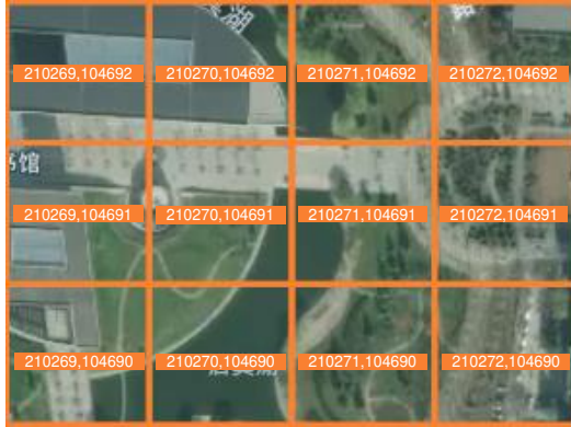
Fig. 4. The 18-level tiles of the Google satellite map in npuchangan . The numbers represent tile information.
