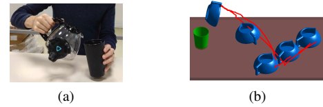
Fig. 5. (a) Human demonstration of a pouring motion using a teakettle to which an HTC VIVE tracker is attached. (b) Visualization of the first trial within a batch of six trials in the same simulation environment as Fig. 4.
