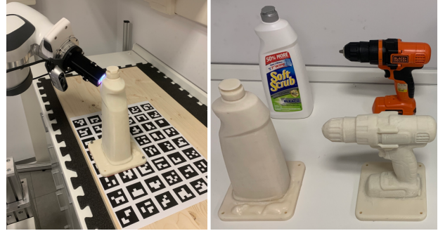
Fig. 5. On the left: the testing setup with the DIGIT sensor touching the “bleach cleanser” object. On the right: example of YCB objects and their 3D printed counterparts.
