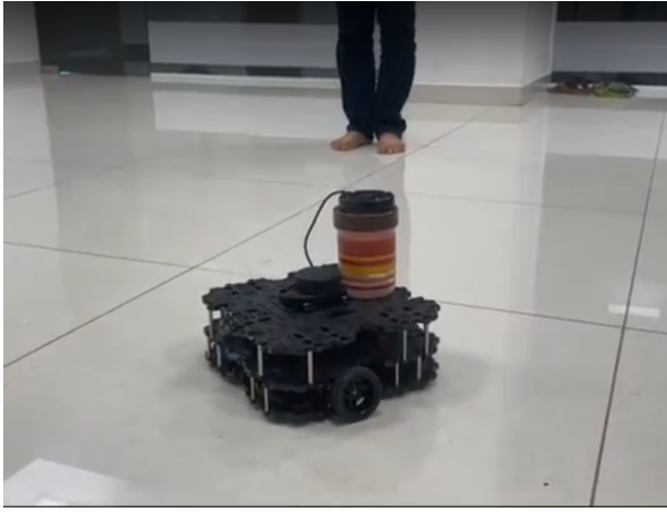
Fig. 4. Mounting of 4-channel circular array microphone on the Turtlebot3 Waffle Pi mobile robot.
