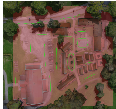
Fig. 4: Top-down view of the Village area. The red bounding box illustrates the volume to be explored. The area is roughly 1 hectare and populated with multiple dynamic obstacles. The paths of the dynamic obstacles are highlighted in green where the lines indicate that the dynamic obstacle moves back and forth while a loop indicates that the dynamic obstacles circulate.
