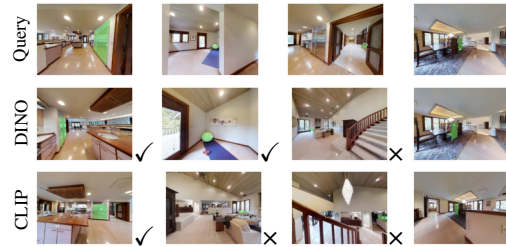
Fig. 3. Object Instance Recognition in GibsonEnv [63]: The rows show segment masks (in green) for the query, DINO match, and CLIP match respectively. Symbols (✓/✗) adjacent to images indicate success or failure in association. The final column illustrates category-level recognition success despite both methods failing at the instance level (multiple chairs in close proximity).
