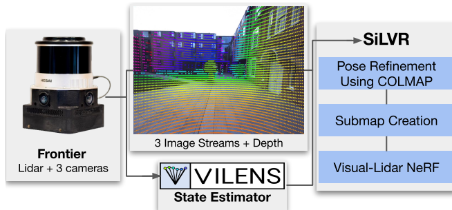
Fig. 2: System Overview: Frontier, our custom perception unit, has three fisheye colour cameras with an IMU and a 3D lidar. Our online state estimator’s trajectory is refined with COLMAP and partitioned into submaps. The camera image, lidar depth, and normal image are used to train a NeRF to get the final 3D reconstruction.
