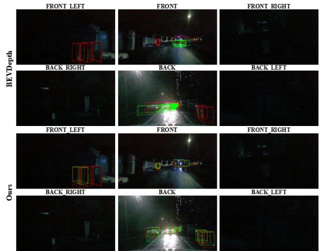
Fig. 4. Qualitative results: The upper and bottom parts are visualization of BevDepth [2] and our proposed method respectively. The results are visualized on the weather adaptation scenario.
