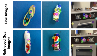
Fig. 3: In each column, given a live image (top) DINOBot retrieves from the buffer the most similar image in the buffer (bottom), and finds correspondences between the two.
