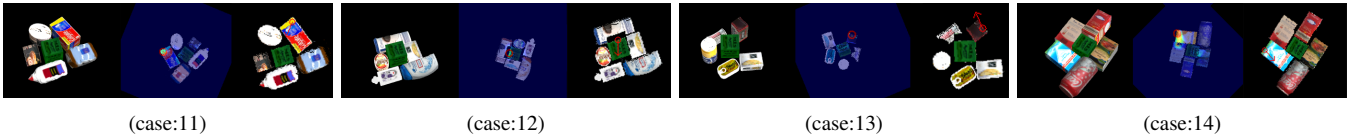
Fig. 7. Four simulated scenes with novel, untrained objects in dense household clutter. The target in each is the green box. The initial column presents the original image; the middle one is the model’s angle and position; the final is the action.
