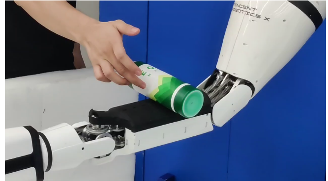
Fig. 1. Stability regulation of a bottle positioned on a robotic arm subject to manual disturbances. Tactile servoing is performed on a custom tactile sensor array covered by black foam on the forearm.
