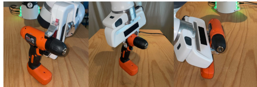
Fig. 4. Example of automatically generated diverse grasps that successfully transferred into the real world.
