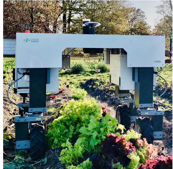
Fig. 1: The autonomous monitoring robot Lero collecting sensor data of a bed in a garden with bio-diverse cultivation
