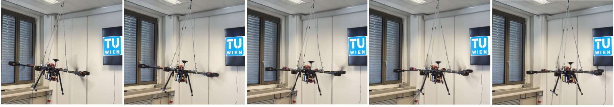
Fig. 9: Sequence of the experiments with the proposed planar-thrust platform being stabilized using the LQR controller.
