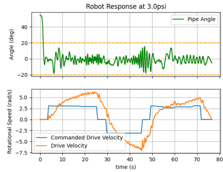
Fig. 12. Experimental Validation of the Driving Controller
