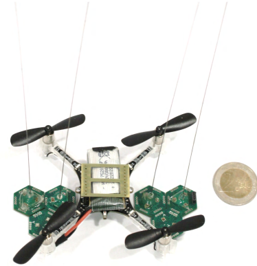
Fig. 1. A size comparison of a tiny UAV ( 92 \times 92 \times 29 mm, 27 g) with a 15 g maximum payload and the proposed whisker sensors ( 20 \times 18 \times 200 mm, 1.52 g).
