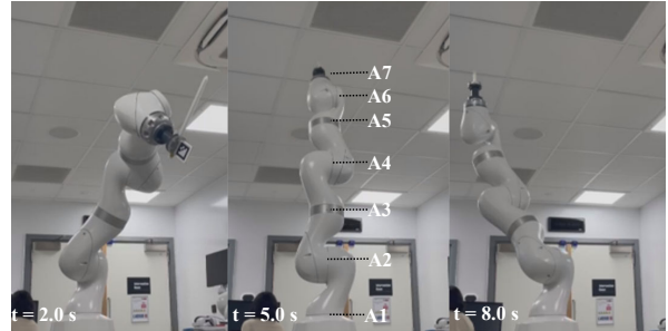
Fig. 1. Snapshots of the trajectory execution for the KUKA LBR Med7 R800 with an EE for different time steps. A1-A7 highlight the individual joints. Our method incorporates the EE's geometry to find trajectories that are collision-free and optimal for dynamic parameter identification.
