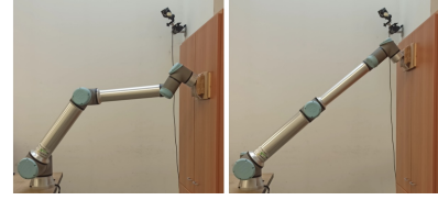
Fig. 4. Impact configurations. On the left, using the propose planner. On the right, using the RRT-Connect planner.
