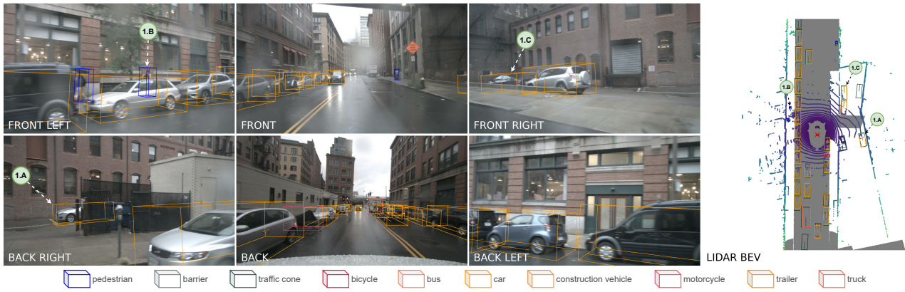
Fig. 5. Example of output predictions with the proposed model on the nuScenes val set. The LiDAR BEV shows ground truth objects in dark green.
