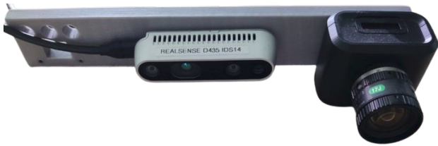
Fig. 4: Sensor setup of the ATIS and Intel Realsense, enabling the development of a synchronized bimodal dataset.
