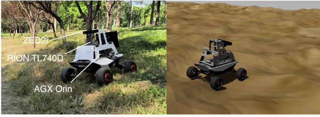
Fig. 4. The mobile robot and corresponding simulator.
