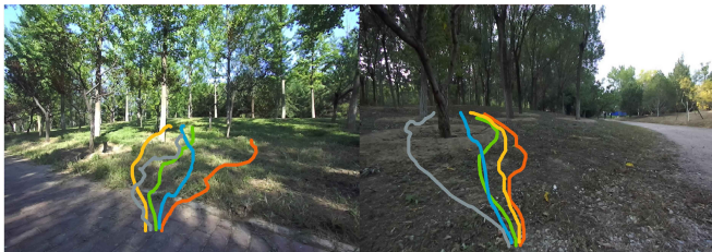
Fig. 6. Trajectories planned by different algorithms in two example scenarios. Our (Green), DWA (Blue), DPC(Yellow), Terp (Grey), BADGR (Orange)
