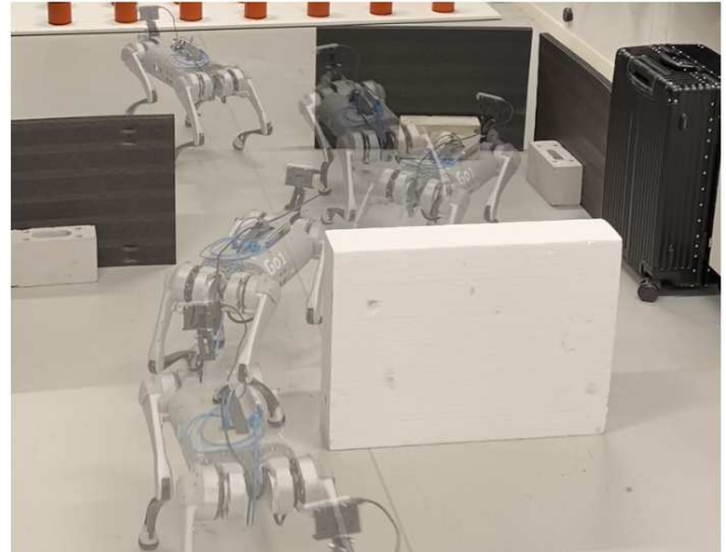
Fig. 1: Visual CPG-RL perceptive locomotion on Unitree Go1.
