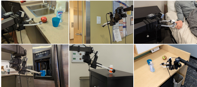
Fig. 4. The real-world experiments consist of 6 picking tasks, 2 placing tasks, a drawer opening task, and a light switch flipping task, encompassing various objects and environments not present in the training set.
