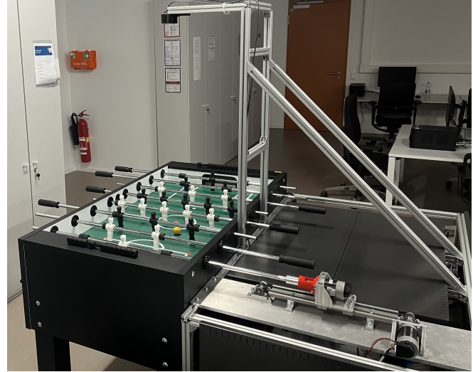
Fig. 1. Our autonomous Foosball system in a human versus machine setting for robust and adversarial robot learning research.
