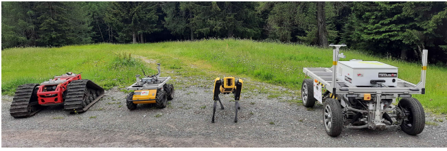
Fig. 4. The four robots used within the experiments. From left to right: Matro Rovo3, Clearpath Robotics Husky, Boston Dynamics Spot, TU Graz Mercator.
