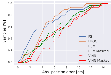
Fig. 6. Position errors between the most suitable demonstration and a query, computed from initial frames. We compare different methods of selecting the best demonstration and observe that the FS function shows the smallest error. We display the cumulative sample numbers satisfying a certain maximum error.
