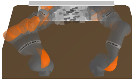
(b) A collection of configurations from a region that represents motions that reach into and out of a shelf.
