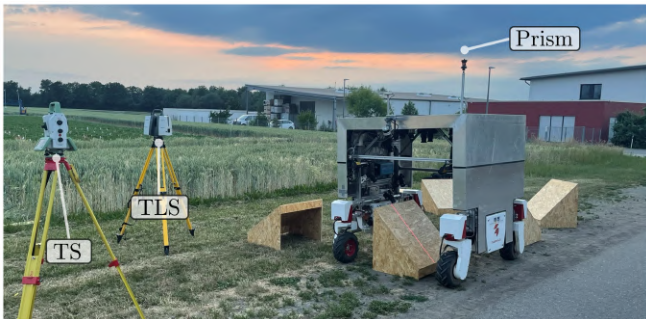
Fig. 3: Calibration test field used to evaluate our calibration approach. The prism is tracked with the Total Station (TS) for precise pose estimation. The Terrestrial Laser Scanner (TLS) is used to create a georeferenced point cloud for calibration and evaluation.
