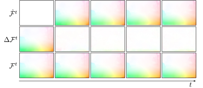
Fig. 3. Initial flow \hat{\mathcal{F}}^t , residual flow \Delta\mathcal{F}^t and final flow \mathcal{F}^t as time progresses and new event bins keeps coming. A trend of increasing quality in \mathcal{F}^t and lowering magnitude in \Delta\mathcal{F}^t can be observed, implying that the flow is iteratively refined through time.
