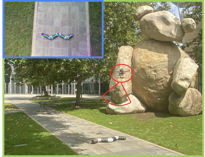
Fig. 1: A snake-like robot, Arcsnake [7], is tracked on camera in the outdoor environment by a hovering drone.
