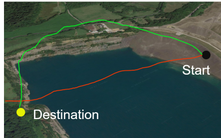
Fig. 1: A drone travels from the start to the destination, crossing a lake. The red trajectory, although shorter, lacks reliable visual features for pose tracking. In contrast, the longer green trajectory enhances visual odometry performance by maximising feature quality over terrain, houses, etc.
