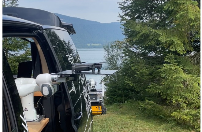
Fig. 1: Concept of mobile hub enabling continuous UAV missions via a robotic arm providing start, landing, maintenance and storage services from inside a vehicle. Off-the-shelf UAVs are able to autonomously start and land on the platform held by the arm at windspeeds up to 5 Beaufort. Between start and landing, the robotic arm can detach the platform and maintain the UAVs.
