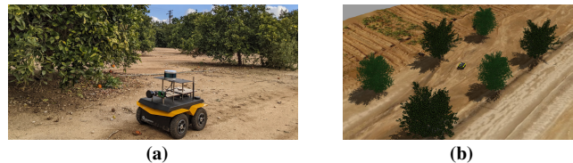
Fig. 1: (a) Clearpath Jackal equipped with a Velodyne VLP-16 LiDAR and a MAPIR Survey3N RGN camera during field experiments. (b) The designed simulation world in Gazebo along with the simulated Jackal mobile robot. This world model contains a 2 \times 3 tree grid of 3 orange and 3 lemon trees placed at a 5 \text{ m} width \times 5 \text{ m} length relative distance from each other.
