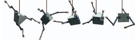
Fig. 4: SpaceHopper reorienting itself to the upright orientation, which is displayed as a black line.
