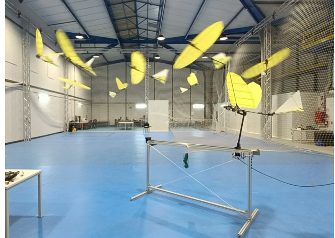
Fig. 1. Trajectory tracking of a circular path; flight of the flapping-wing robot in the test bed environment.
