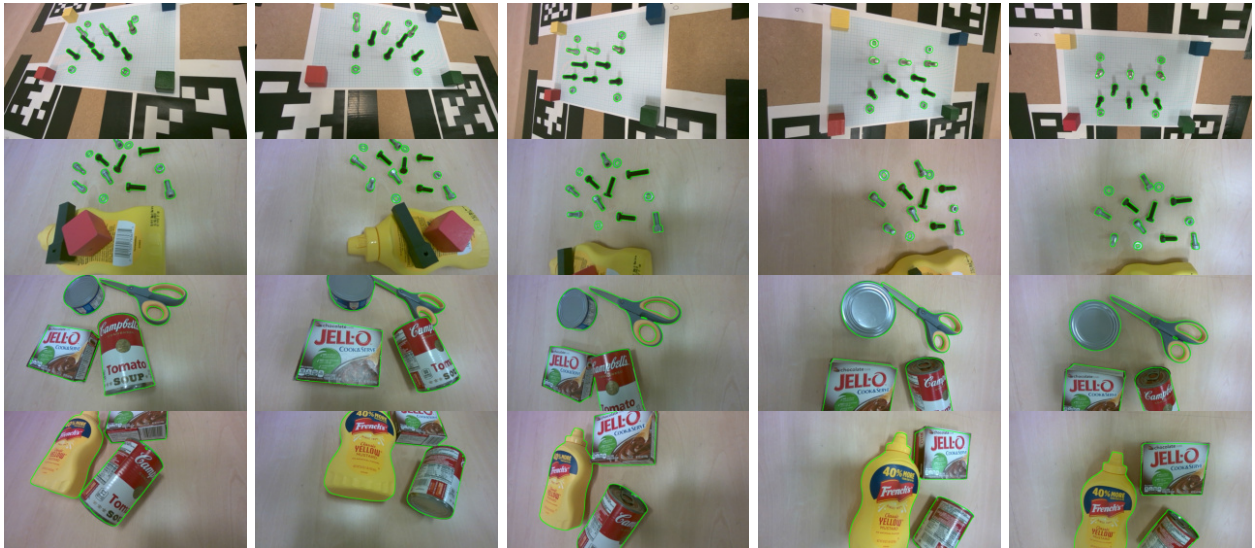
Fig. 4: Self-collected real-world datasets where the poses of all the relevant objects are accurately estimated, as evidenced by the re-projection of the silhouettes of their models perfectly aligning in the image plane.
