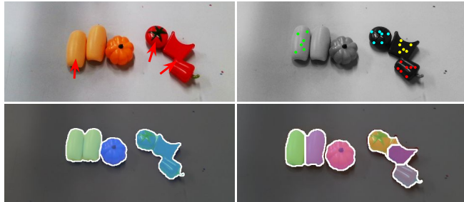
Fig. 1: Interactively segmenting a cluttered scene with minimal, non-disruptive pushes. [Top left] Initial scene and identified robot actions. [Top right] The origins of sampled body frames with matched BFIFs due to scene interactions, where matched body frames share the same color. [Bottom left] Undersegmentation of scene’s end configuration by static segmentation model. [Bottom right] Accurate segmentation of scene by RISeg after interactions have been completed.
