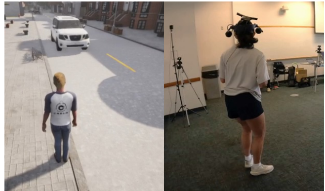
Fig. 2. Example of JaywalkerVR simulation. Left: Subject’s avatar in the JaywalkerVR from a third-person perspective. Right: Captured image of a subject wearing the VR headset in the data collection environment in the real world.
