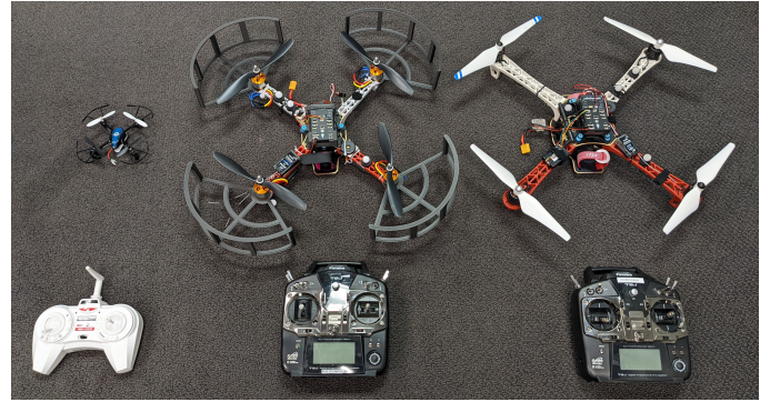
Fig. 2: Holystone HS170 mini UAV was used with the white RC, and Flamewheel F330 (with prop-guards) and Flamewheel F450 were used with the Futaba controller.
