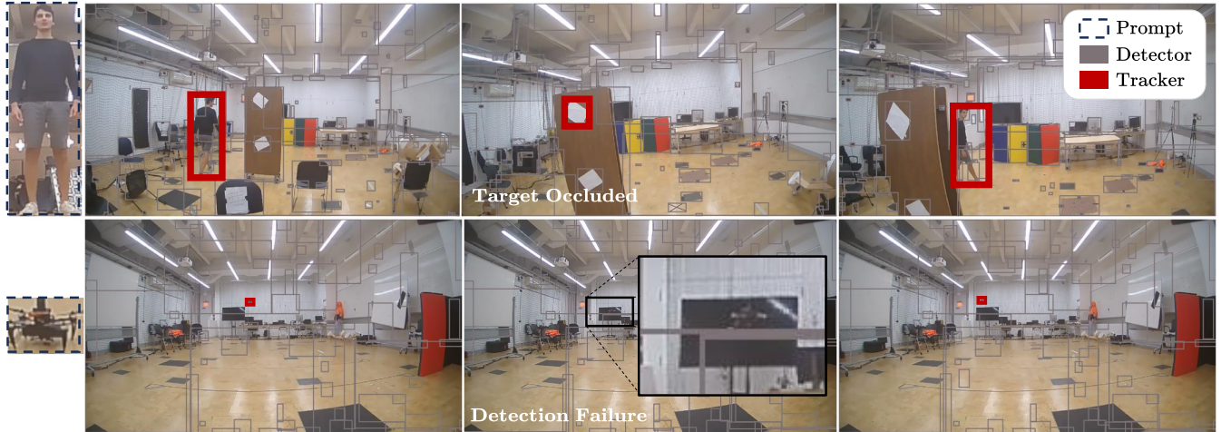
Fig. 4: Our detection and tracking algorithm’s resilience and accuracy. Top row: Indoor spatial-temporal tracking of a human against occlusions. Bottom row: Tracking of our custom-made drone, highlighting re-identification capabilities.
