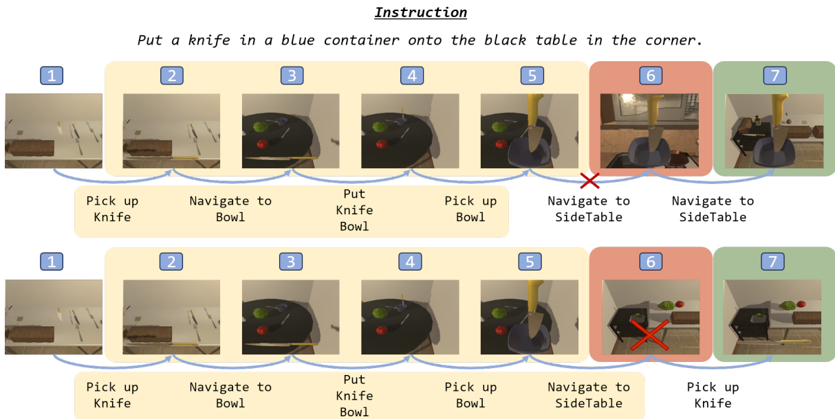
Fig. 3. Illustration of re-planning procedure This figure illustrates the re-planning procedure. In both rows, the agent performs four actions following the high-level instruction: picking up the knife, navigating to the bowl, putting the knife in the bowl, and picking up the bowl with the knife. In the first row, an erroneous navigation occurs, leading the agent to the microwave. In the second row, a manipulation error results in the agent dropping the bowl and knife.
