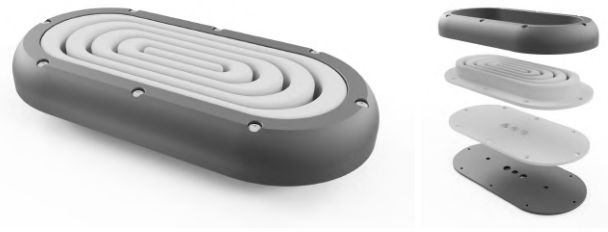
Fig. 2: An individual telescopic structure of the proposed soft robotic sun tracking mechanism. Left subfigure shows an assembled telescopic structure. Right subfigure shows an exploded view of the telescopic structure assembly's four main components.
