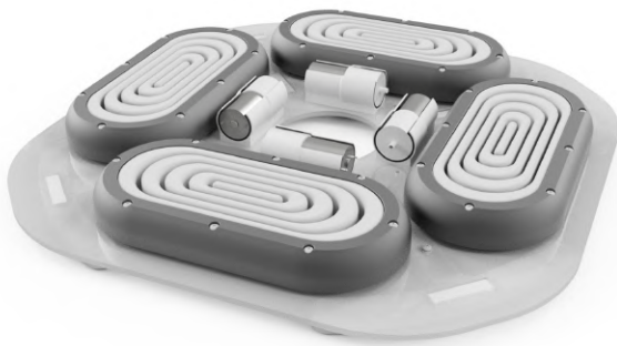
Fig. 4: The bottom platform assembly as a 3D CAD render. Four telescopic structures are arranged in a ring on an acrylic base surrounding the four air pumps used to pneumatically actuate them.
