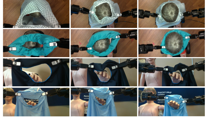
Fig. 4: Snapshots during four real-world dressing scenarios. Our controller successfully inserts the openings by taking advantage of the contacts between the garment and the body.
