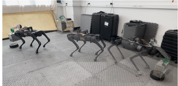
Fig. 1: Snapshots of Aliengo lifting and carrying a 5kg payload. Supplemental video: https://youtu.be/0hYDa94F78E
