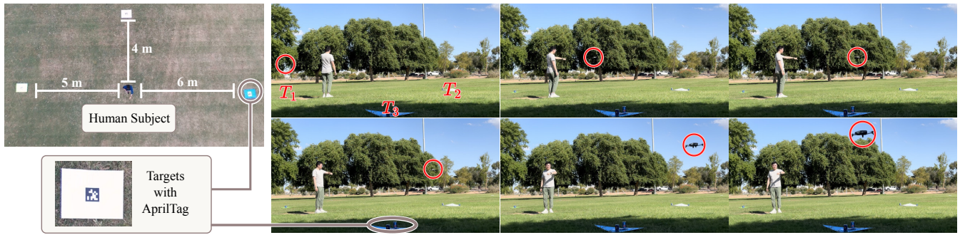
Fig. 7. Left: The drone piloting task setup. Targets ( T_1, T_2, T_3 ) were marked with AprilTags [29] to be detected through the camera stream of the drone. Right: Human subjects piloted the drone to all three targets in a given random order. This figure depicts the control with iRoCo, where the user only had to point toward the target and adjust elevation and distance with their wrist.
