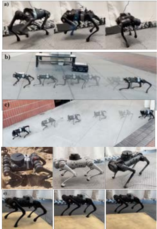
Fig. 1. Experiment result highlights. a) High-speed steering in place; b) High-speed running; c) High-speed running and steering; d) Generalization of the same policy across different robot platforms; e) Transition between soft and hard terrain. Experiment video: https://www.youtube.com/watch?v=HxSIxTnEw08
