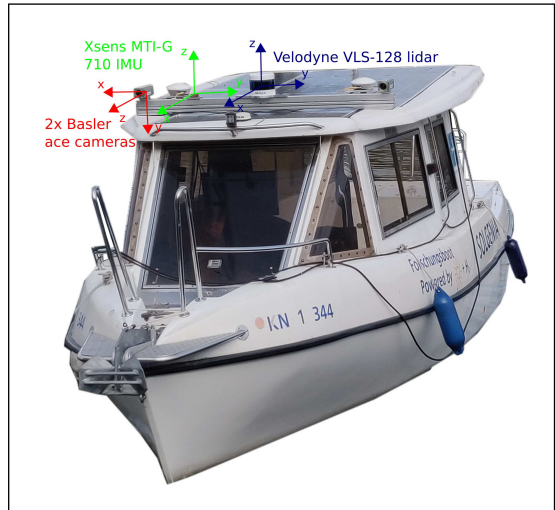
Fig. 2. The research vessel “Solgenia” equipped with two RGB cameras, a laser scanner, and an IMU.
