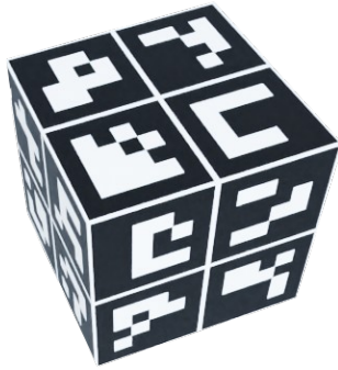
Fig. 4. Cube with side 0.575m covered in 24 ArUco markers with side 0.276m, used as the dynamic object in the bipartite pose graph.
