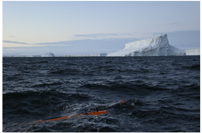
Fig. 2. Kongsberg’s Hugin AUV (orange) during the recovery of a survey in West Antarctica.
