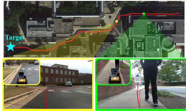
Fig. 1: Trajectory generation in a campus environment. The top view is the robot’s trajectory (around 350m). The bottom row shows generated trajectories at the two locations corresponding to green and yellow boxes, respectively. The trajectory closest to the global target, shown at the top, will be chosen to provide waypoints for the local planner. The local planner drives the robot and avoids collisions [7]. In this complex outdoor scenario, our MTG global navigation method can efficiently and safely generate trajectories for global navigation and cover most of the traversable areas, including the narrow pedestrian sidewalks.
